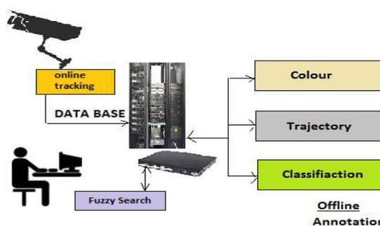
Figure 4: Architecture of VIGILANT surveillance system [21]
