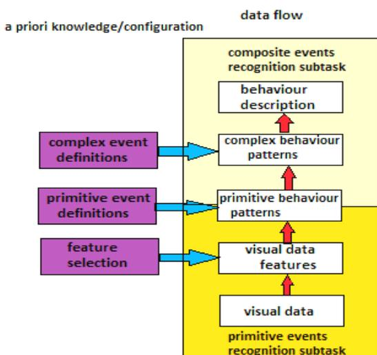
Figure 1: Generalized architecture of visual surveillance system [18]
