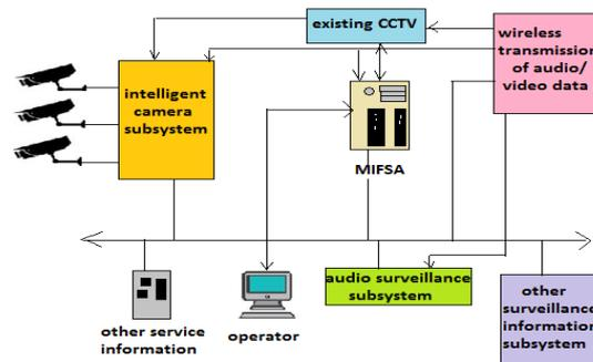
Figure 3: Architecture of PRISMATICA surveillance system [20]
